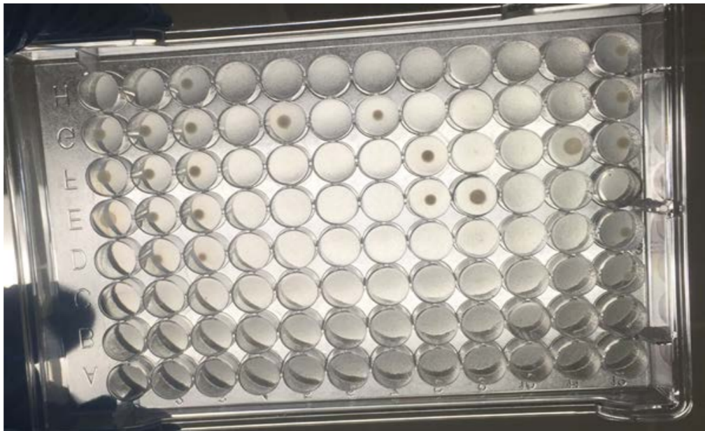
Figure 5. Sensititre® plate post inoculation and incubation. Accumulation in well indicates resistance
